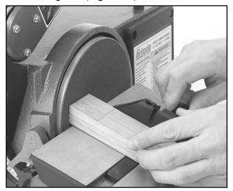
Figure 19. Mitering with the table angled.
